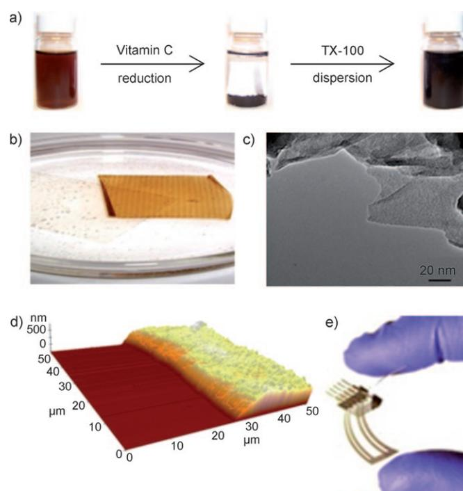
**Figure 1.** (a) Digital images of the vials containing GO and RGO dispersions. (b) Inkjet-printed graphene oxide film lifts off the PET surface. (c) TEM image of the RGO powder. (d) AFM image of RGO film obtained by reduction of the film in (b) with ascorbic acid. (e) Digital image of inkjet-printed RGO/PET four-probe sensor.
