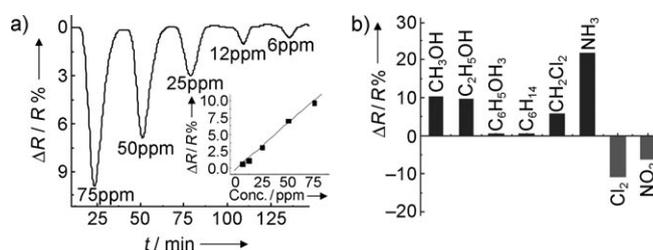
**Figure 3.** Vapor sensing by inkjet-printed RGO/PET obtained by ascorbic acid reduction of dispersed graphene oxide. (a) Plot for resistance versus time when the film was exposed to a  $\text{Cl}_2$  vapor. Inset: Plot of resistance versus vapor concentration. (b) Selectivity plot: sensor exposed to saturated organic vapors,  $\text{NH}_3$  (100 ppm),  $\text{NO}_2$  (100 ppm), and  $\text{Cl}_2$  (100 ppm).
