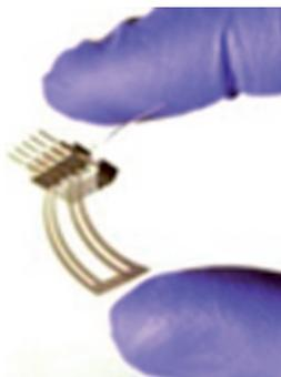
**Flexisense:** Films of graphene oxide and reduced graphene oxide are printed onto a flexible plastic surface (see picture), using inkjet techniques, which are used to detect chemically aggressive vapors such as  $\text{NO}_2$  and  $\text{Cl}_2$ . Vapors in the 100 ppm–500 ppb concentration range can be detected in an air sample without the aid of a vapor concentrator.
