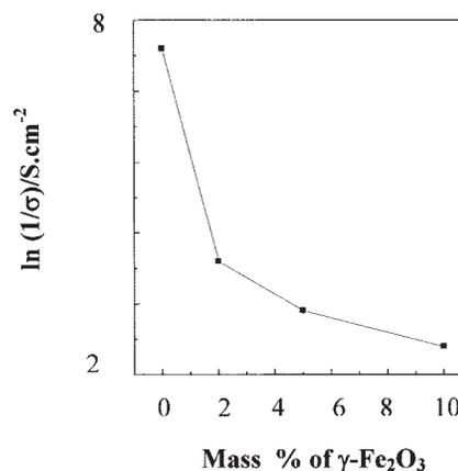
Figure 6 Conductivity versus mass %  $\gamma$ -Fe<sub>2</sub>O<sub>3</sub> loaded in nanocomposites.
